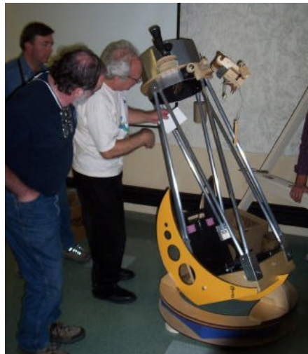
Stargazer Steve Dodson demonstrated his unique telescope design at a recent meeting of the Peterborough Astronomical Association. At 13" aperture, it is a large scope. But it all breaks down and can fit into a mini-sized car with ease.
